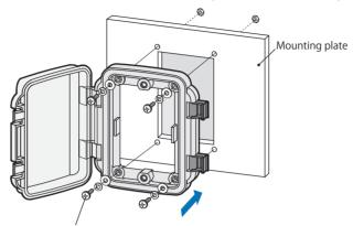
Round head screws: 4xM4 (not supplied) Frame thickness of screw hole 5mm (0.20 in.) Tightening torque: 0.5 to 0.7 N·m (4.4 to 6.1 lb-in.)
